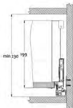
Drawer slide installation dimensions
